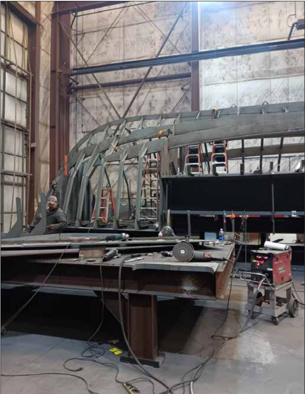
A closer look at the bow of the R/V Steelhead II. The vessel will replace the DNR's current research vessel which has been in operation for over five decades. (Courtesy/Sarah George)
