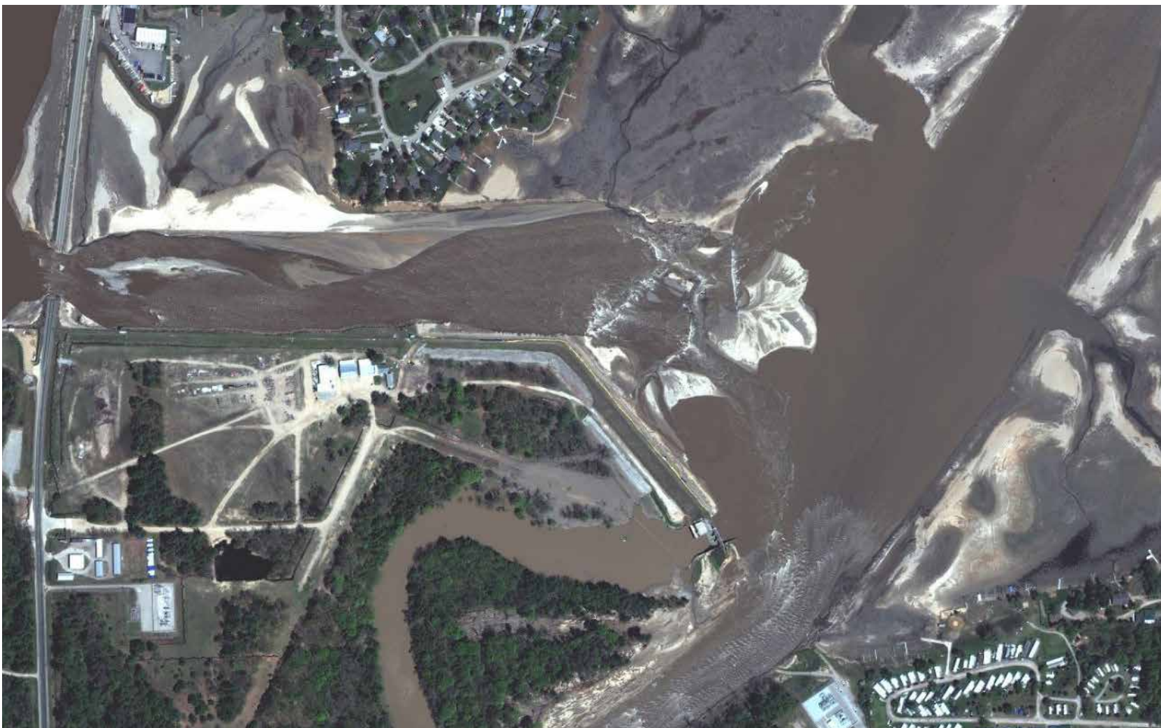
The Midland dam failures of 2020 flooded out a large swath of mid-Michigan, causing widespread damage after a parade of owners over decades failed to adequately maintain and upgrade the dams. (Bridge file photo)
