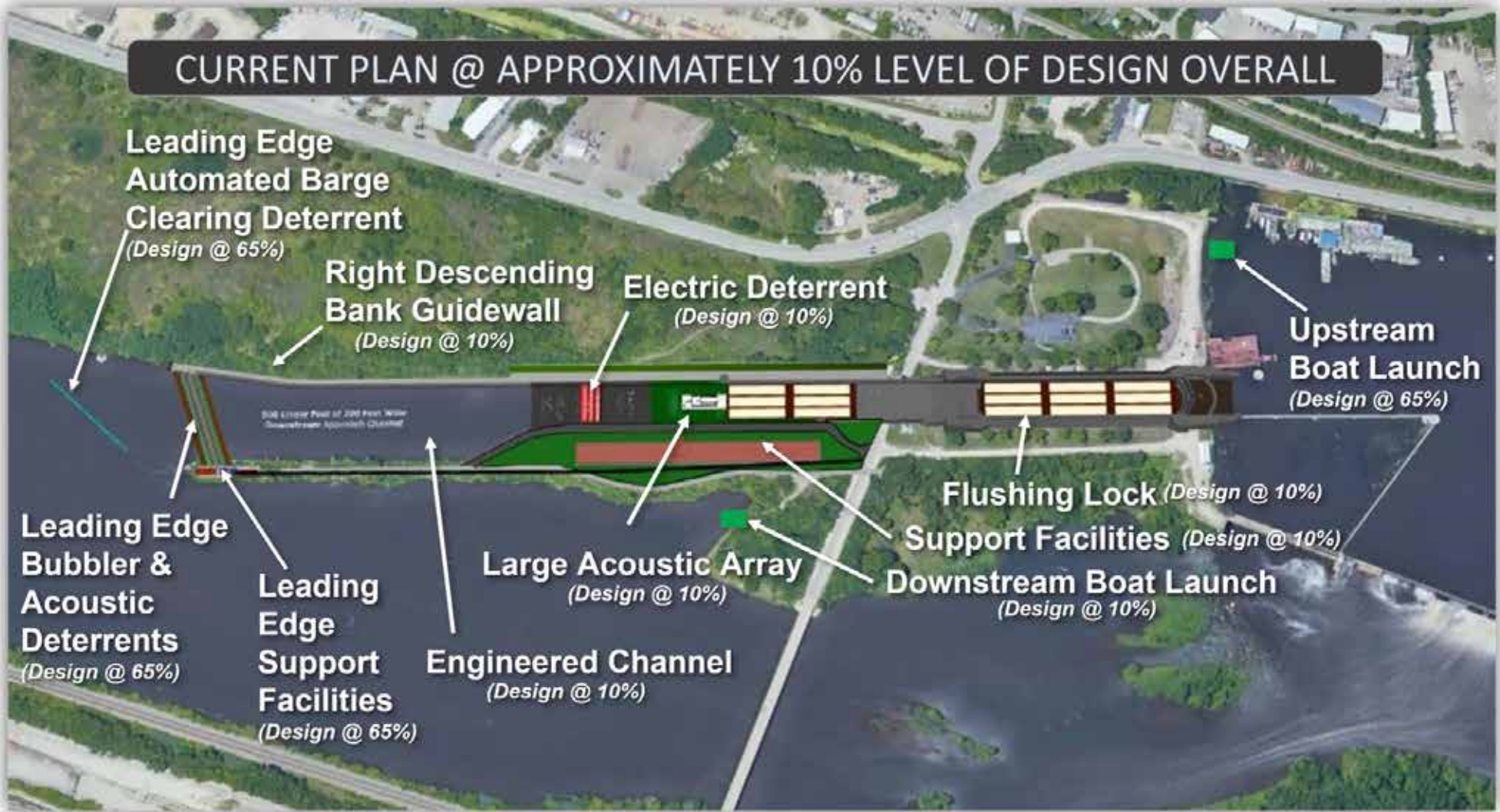
The new Brandon Road invasive carp barrier design issued December 2022. Photo credit: USACE
